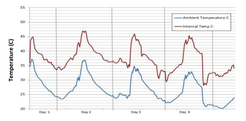
The thermal test performed on field, confirms a maximum internal termperature below 50 C, even with summer environmental temperatures.
