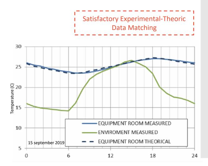
These recorded data has been analized through Celantel thermal simulator software.
